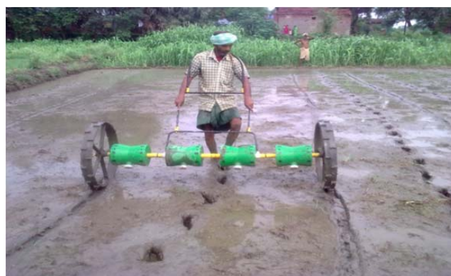
Field operation of 8 row paddy seeder in puddle condition
